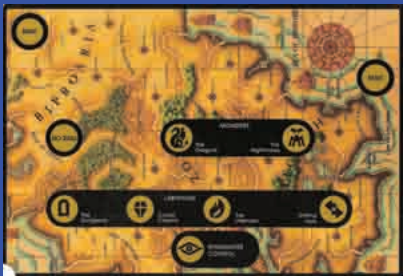
» This thin plastic overlay was placed over the membrane keyboard to change it into a control panel for the on-screen action.
